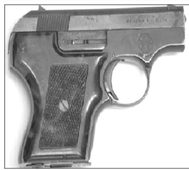
Below left: The S&W 422/622 and derivatives trace their basic design concept to the 1908 Pieper Bayard pistol, which featured the recoil spring over the barrel and the recoil spring guide “keyed” to the slide by the removable front sight assembly. Below right: The familial predecessor to the Models 422/622 was the short-lived S&W Model 61 Escort of the early 1970s. Compare the Model 61 to the 1908 Bayard—the ejection port and extractors appear strikingly similar.
