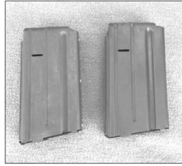
Left: The 17DM-180 lower receiver is machine to accept the ubiquitous AR-15/STANAG magazine, unlike the two original AR-180 magazines with their narrow mag catch slot on the right side of the magazine as shown.
