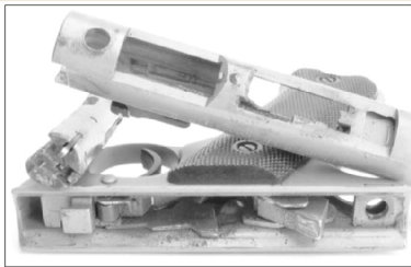
Above: The "after" results (right) from ultrasonic cleaning can be dramatic, as demonstrated by this suppressed Ruger Mark II Amphibian by AWC.
