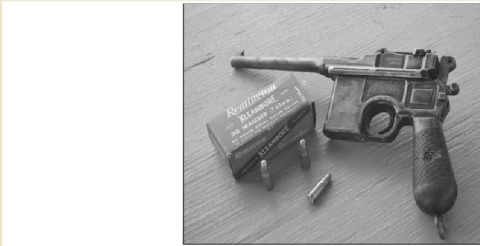
Left: While a number of variations and chamberings exist, the classic C96 is chambered in 7.63x25mm Mauser (.30 Mauser) with a fixed tenround magazine.
