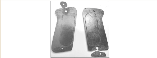
Left: The Bakelite grips, showing the spalling at the screw holes. Baxter went to his go-to solution in such cases—J-B Weld.
