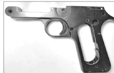
Below: Left side of the Reising frame with the grips off, exposing the operation of the sear bar and the sear spring.
