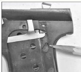
Left: No. 2 pencil points to the firing pin which has been inserted into the hole slightly beneath the trigger bar following compression of the hammer spring with an awl or other tool. The firing pin keeps the hammer plunger and hammer spring compressed and removes force from the hammer strut, allowing the hammer pin and hammer to be removed. The hammer is shown in the forward position, ready for its axis pin to be pushed out.
