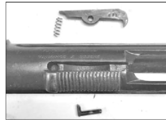
Left: The extractor and spring are shown removed from the slide with the short L-headed retaining pin beneath the slide. Note that the extractor is serialized.
