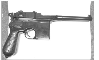
Below left: The left side of the finished product. Remarkably, the Chinese characters on the left side of the magazine well that were very faint originally were actually enhanced by the application of Lauer's Dura-Coat. Below right: The right side of the finished product. The finish, prepared with careful sanding and J-B Weld, is nicer than the original.
