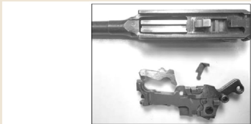
Below left: The barrel/receiver and action when removed from the frame. The action unsnaps from the barrel. Below right: The action removed from the barrel. The bolt locking block will come off and either the sear, the lock frame stop, or both will probably fall out.
