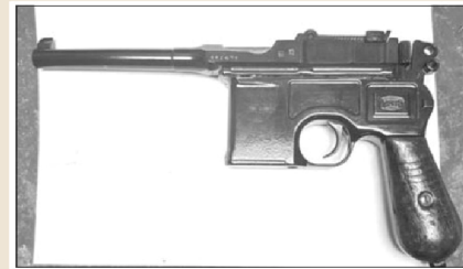
Below left: The left side of the finished product. Remarkably, the Chinese characters on the left side of the magazine well that were very faint originally were actually enhanced by the application of Lauer's Dura-Coat. Below right: The right side of the finished product. The finish, prepared with careful sanding and J-B Weld, is nicer than the original.
