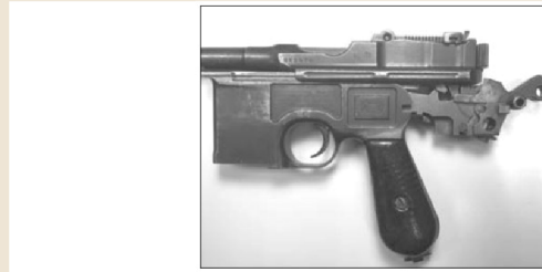
Far left: The pistol aligned to be taken down. The lock frame stop is at the top of the backstrap under the hammer. Left: The barrel/receiver and action sliding out the back of the frame.
