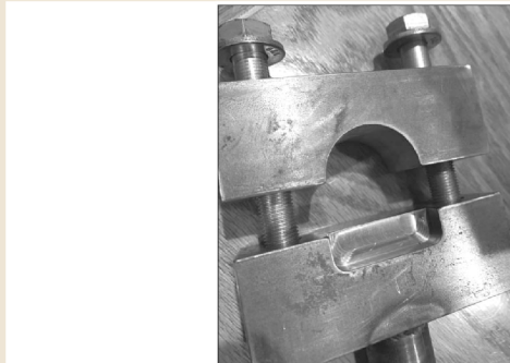
Left and above: An assembled wrench. Here we see the half round for the receiver ring, the bolts used to squeeze the ring, and the cutout for the recoil lug. You can also see the handled welded on. The other end is aggressively knurled for grip texture. This setup worked remarkably well! ORIGINAL ARCHIVE IMAGE · PERMISSION CONFIRMED
