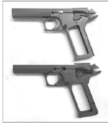
Left: Ignoring distortion from the camera wide-angle lens, the P210 Standard (and Target) frame (top) is identical to that of the P210 Carry (bottom). ORIGINAL ARCHIVE IMAGE · PERMISSION CONFIRMED
