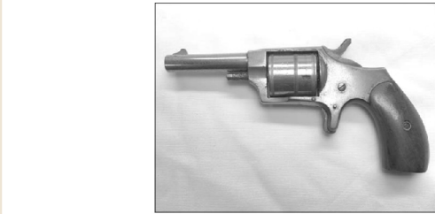
Right: Spur trigger H&A models are represented here by the Dictator in .32 RF. It is a bare bones singleaction revolver with a nickelplated cast iron frame, walnut grips, and a five-shot cylinder.
