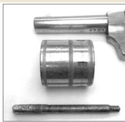
Below left: Example of the H&A folding hammer spur available as an option on some models to facilitate pocket carry and draw without the hammer spur catching on clothing. Below center: The paddle-shaped cylinder axis pin release is a telltale for H&A-made revolvers of the Forehand & Wadsworth design. Below right: Demounting the cylinder is easy. The cylinder axis pin is left-hand threaded and features a thin slot at its forward end. Remove the pin and the cylinder literally falls out to the right; there's no loading gate.
