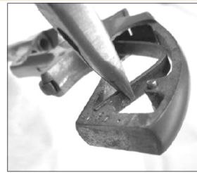
Left: Lower end of mainspring being placed into its seat in the frame using pliers.
