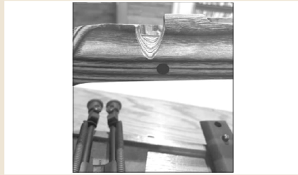
Left: The finished bolt channel.
