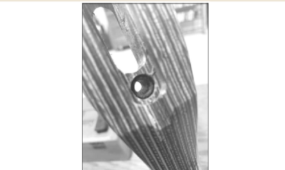
Below left: Rear action screw ferrule installed in the stock. I will still need to glass bed it in place. Below center: The front ring/recoil lug pocket after opening it up to fit my receiver. Below right: The trigger slot has been slightly elongated to allow for a clearance fit of the adjustable trigger unit that comes with the receiver.
