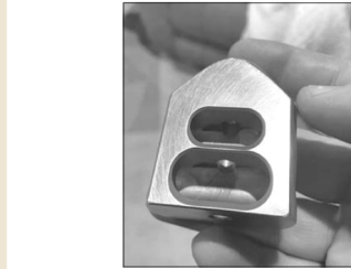
Above and left: The custom muzzle brake I machined and finished out of a chunk of stainless steel I had laying around shown from different angles.
