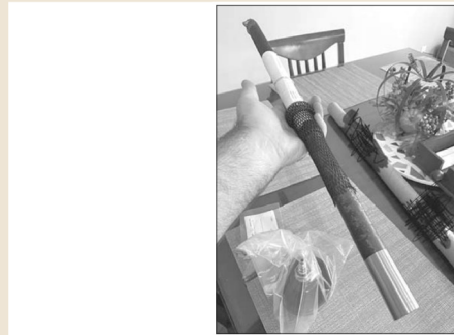
Above: The carbon fiber-wrapped barrel from Carbon Six. It is ready to be threaded and fitted to the M98 action.
