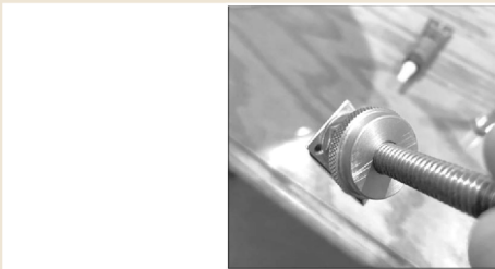
Left: The old Weaver ring machined and the allthread attached. The brass lock nut as machined, ready for assembly.
