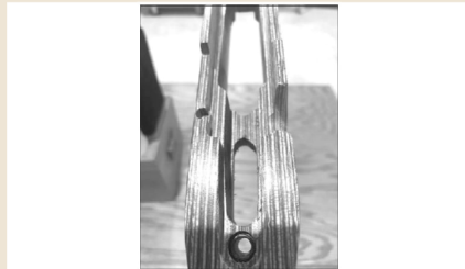
Below left: Rear action screw ferrule installed in the stock. I will still need to glass bed it in place. Below center: The front ring/recoil lug pocket after opening it up to fit my receiver. Below right: The trigger slot has been slightly elongated to allow for a clearance fit of the adjustable trigger unit that comes with the receiver.
