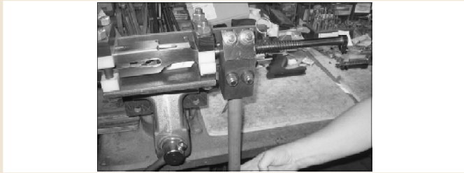
Right: Here, the Richardson Universal Barrel Wrench is positioned with the receiver clamped in a special vise.
