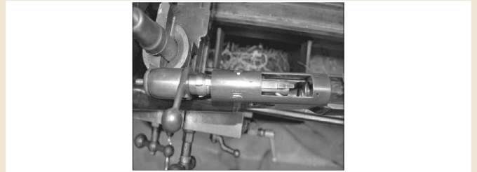
Below: Detail of the Vetterli action with the new bright yellow firing pin assembly. Note how the bolt locks at the rear by rotating the handle as the body stays still.
