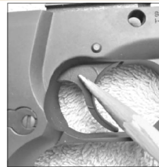
Left: The absence of a cross pin in the area of the trigger indicated by the No. 2 shows that the SA-35 is produced without a magazine release. If present, the pin retained the slotted shaft of a spring-loaded plunger that made contact with the magazine and allowed the trigger to rotate to the rear, tripping the sear.
