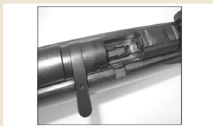
Far left: Olympia carbine shown in battery, illustrating the butter knife bolt handle, receiver ring with two scope mount screw cross grooves, and massive adjustable rear sight. Left: Olympia rifle action shown open, with the bolt handle locked into the rear notch. The forward bolt handle notch is clearly visible, along with the breech end of the barrel and the top of the empty magazine.
