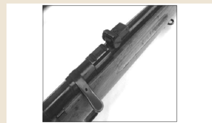
Far left: Olympia carbine shown in battery, illustrating the butter knife bolt handle, receiver ring with two scope mount screw cross grooves, and massive adjustable rear sight. Left: Olympia rifle action shown open, with the bolt handle locked into the rear notch. The forward bolt handle notch is clearly visible, along with the breech end of the barrel and the top of the empty magazine.
