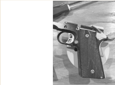
Left: Attaching the grip panels back onto the pistol using the new grip screws from Brownells. ORIGINAL ARCHIVE IMAGE · PERMISSION CONFIRMED
