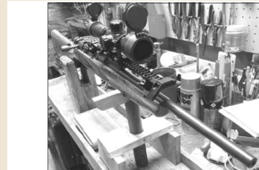
Below: The rifle from the back. This shows the orientation of the offset iron sights and the height of the scope, which turned out to be okay for cheek weld. Below right: The rifle from the front. The cantilever and offset iron sights are a bit jarring to the traditional mind, but they work.
