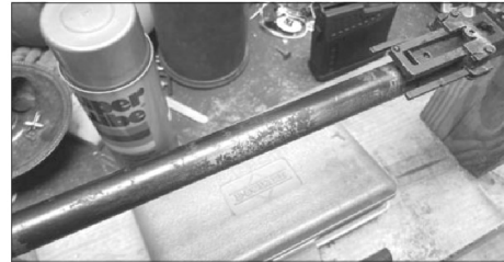
Right: The barrel showing light pitting and the anti-aircraft rear sight.
