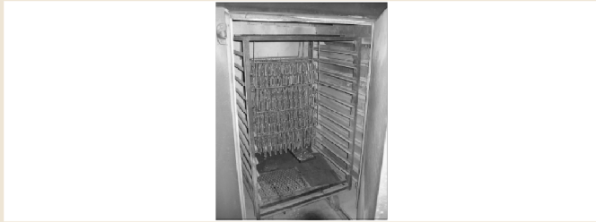
Right: After autocatalytic plating, parts are rinsed in deionized water and then given a stress-release heat treatment in an oven at 220 degrees F.
