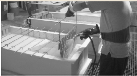
Below: A Robar employee removes and rinses off a rack of freshly plated parts from the autocatalytic plating bath.
